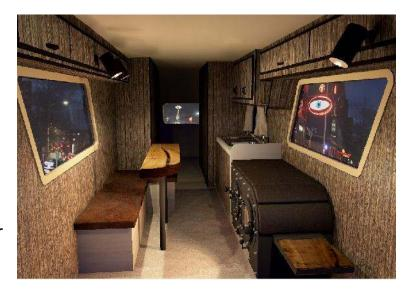
The presented stove is a pure radiant heater, as for that not only the producing heat, but also "her" firetube look is radiant. The heated gas from the burner US goes sidewise into a baker module and then out to the chimney. The stove is covered in sandblasted steel plates and has a ceramic bench on top of it.
