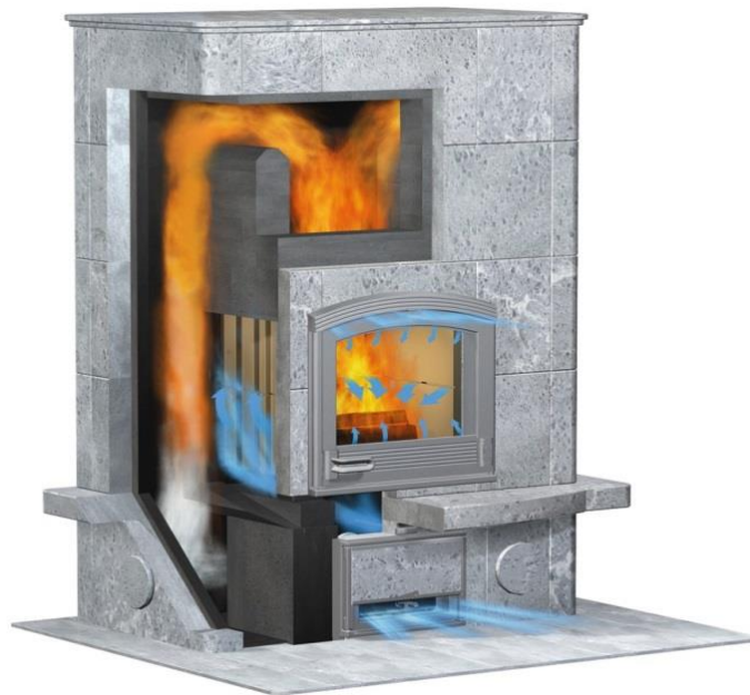
Figure 4: Typical path of flue gases through a Contraflow Masonry Stove. The point of entry to masonry channels is at a temperature of approximately 650C
