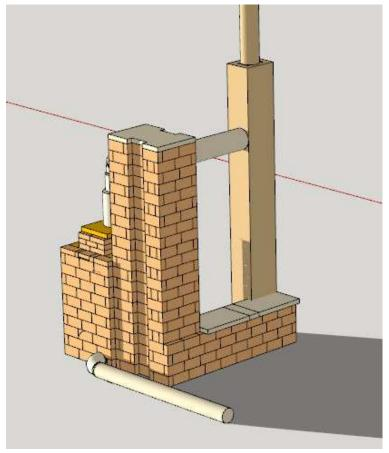
The gases exit into a heated bench that connects to the chimney. The pipe in front is for measuring the intake air flow.
