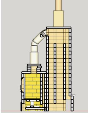
The existing version, above, has 3 parallel downdrafting channels. In configuration #2, we will downdraft the first channel, updraft the second, and downdraft the third.
