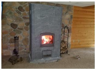
From an emissions point of view, masonry heaters have always been clean burning. This is not due to elaborate firebox designs but rather to the way combustion is conducted: at a high burn rate, typically 10 times higher than in a wood stove. Smoldering never occurs.
