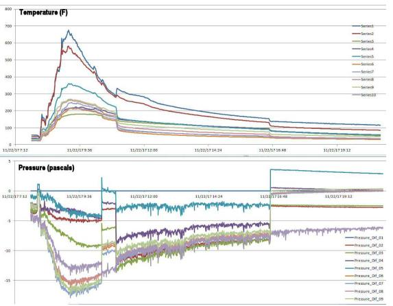
Not obvious is pressure sensor 1, which is in free air, with no differential pressure. It is the dead flat blue line at 0.
