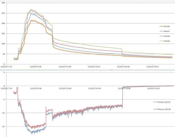
The timeline is over about 12 hours, opening the chimney damper and lighting the heater at 8:00 am and closing the chimney damper 100% at around 4:30 pm.
