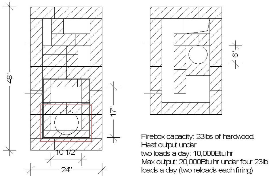
We are starting with this multi-functional heater to show an alternative to the classic rocket stove, however, options for designs are endless starting from very small room heaters to very large with heated benches and other functions. Here are quick design sketches for a couple of other possible layouts:
