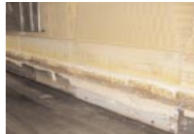
Emisshield™ coated steel kiln car skirts resist oxidation and warping
