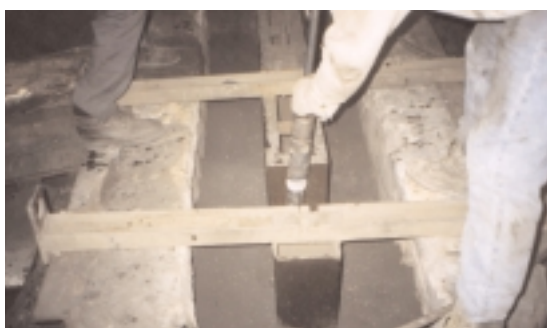
Installation of RAMAL 85 G in cupola trough application.
