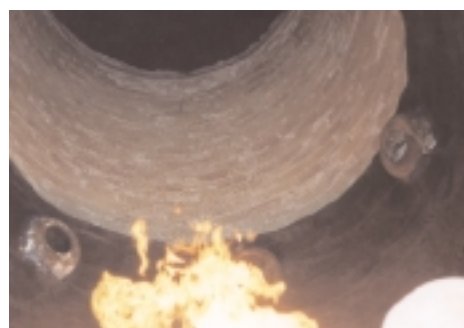
NARCARB ZP Plastic lining a cupola well zone
