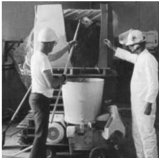
Here you can see the BSM Gun, the "V" Shaped opening in the bulk carton, and the GREENGUN® plastic being raked into the hopper.
