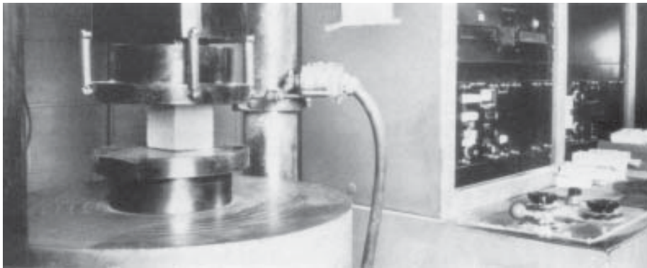
Figure 3.1 Cold Crushing Strength Test
