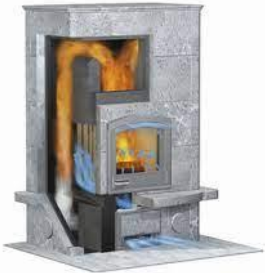
Schematic of factory-built, site assembled, soapstone masonry heater
